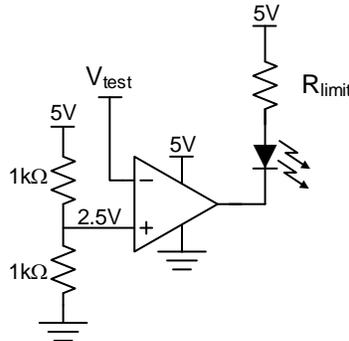
Figure 1: Example comparator circuit that turns on the LED when  $V_s > 2.5V$
