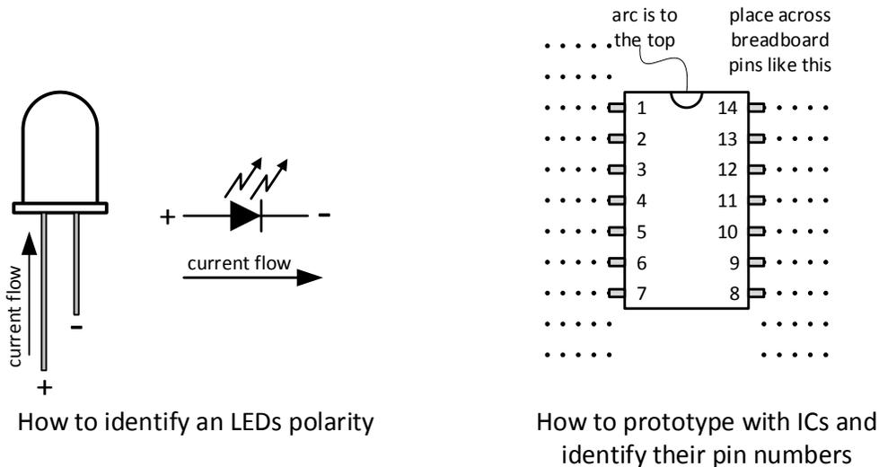
How to identify an LEDs polarity
