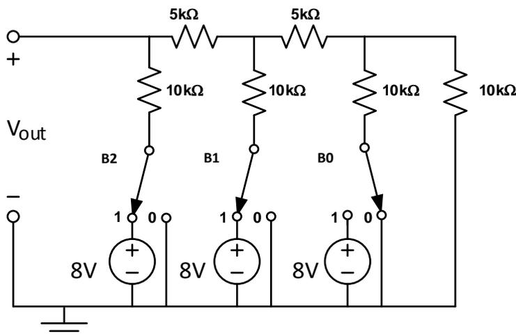
Figure 2 – D/A Converter Circuit. The switches are set to 110 binary (110 means B2=1, B1=1, B0=0) and are read left to right with the most significant bit on the left.
